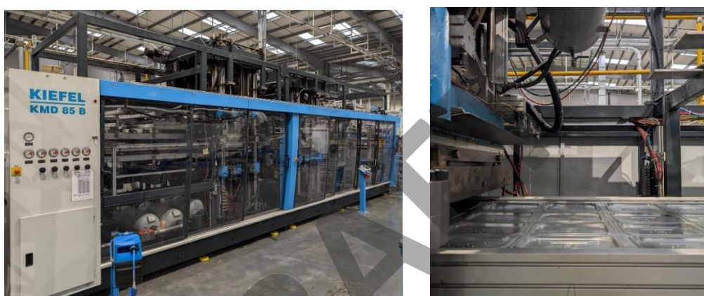
Figure 3.25. Dawn meats' thermoforming Kiefel KMD 85 B machine.
