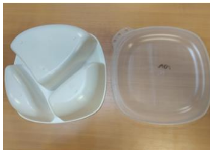
Figure 3.3. Vytal three compartment developed under BUDDIE-PACK project. Injected part by CADPRO during tuning process (01/25).
