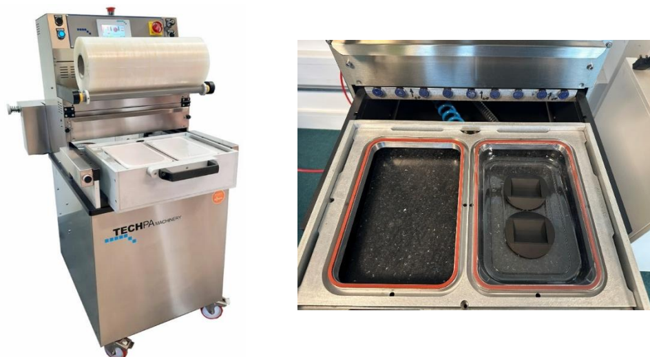
Figure 3.29. Left: Techpa TM50 Skin vacuum sealing machine. Right: internal machine bed for tray placement.
