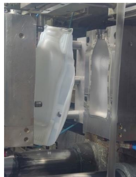
Figure 3.5. Asevi's bottle production.
