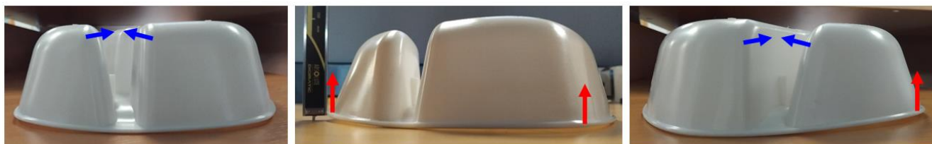
Figure 3.4. Vytal prototypes under tuning process: flatness deformation given by geometrical stresses.
