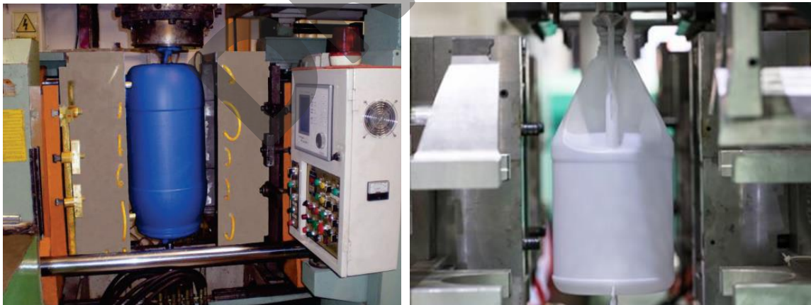
Figure 2.3. Extrusion blow moulding example.
