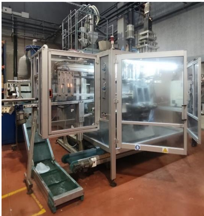
Figure 3.8. Asevi's extruder Magic Machine model ME-L8-10/ND
