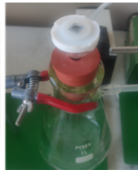
Square silicon membrane set in the vacuum filtration unit to collect microplastics
